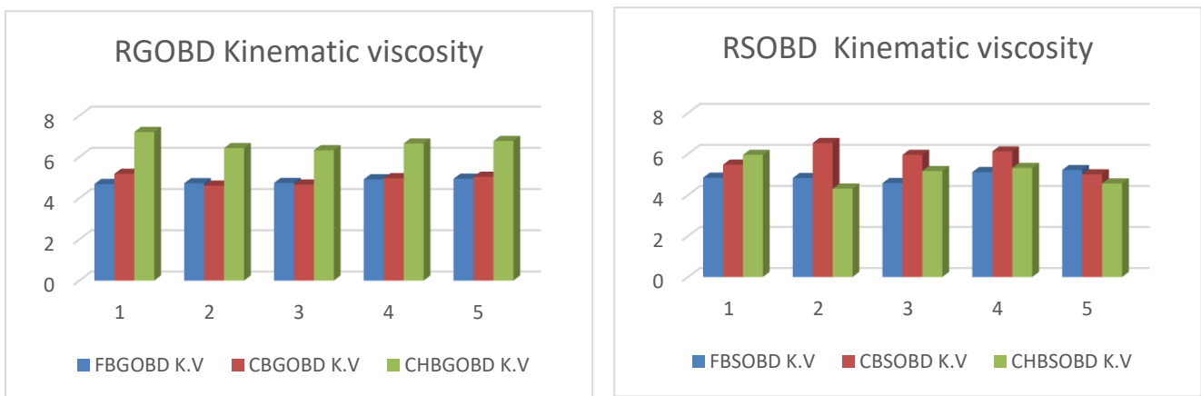
Figure 8 The effects of catalyst dosages on the kinematic viscosity of RSOBD and RGOBD
