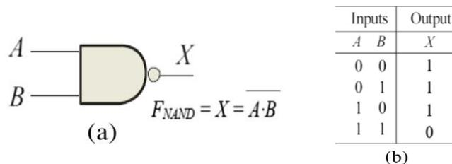
Figure 4 (a) NAND logic gate symbol, and (b) NAND logic gate truth table
