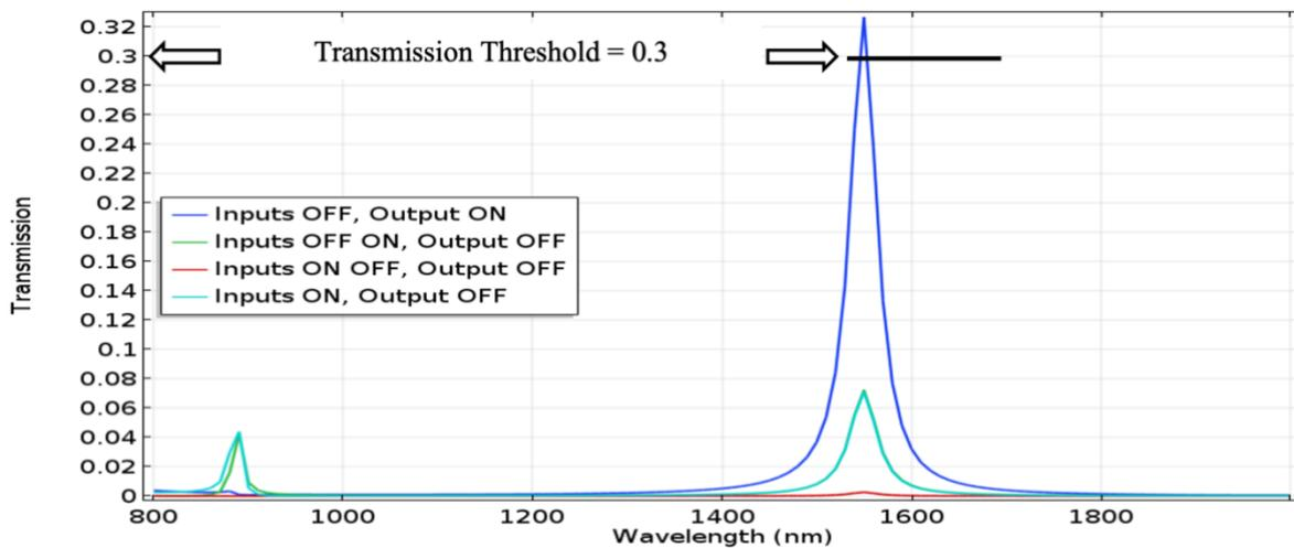
Figure 3 The transmission curve Vs. the wavelength range for NOR logic gate
