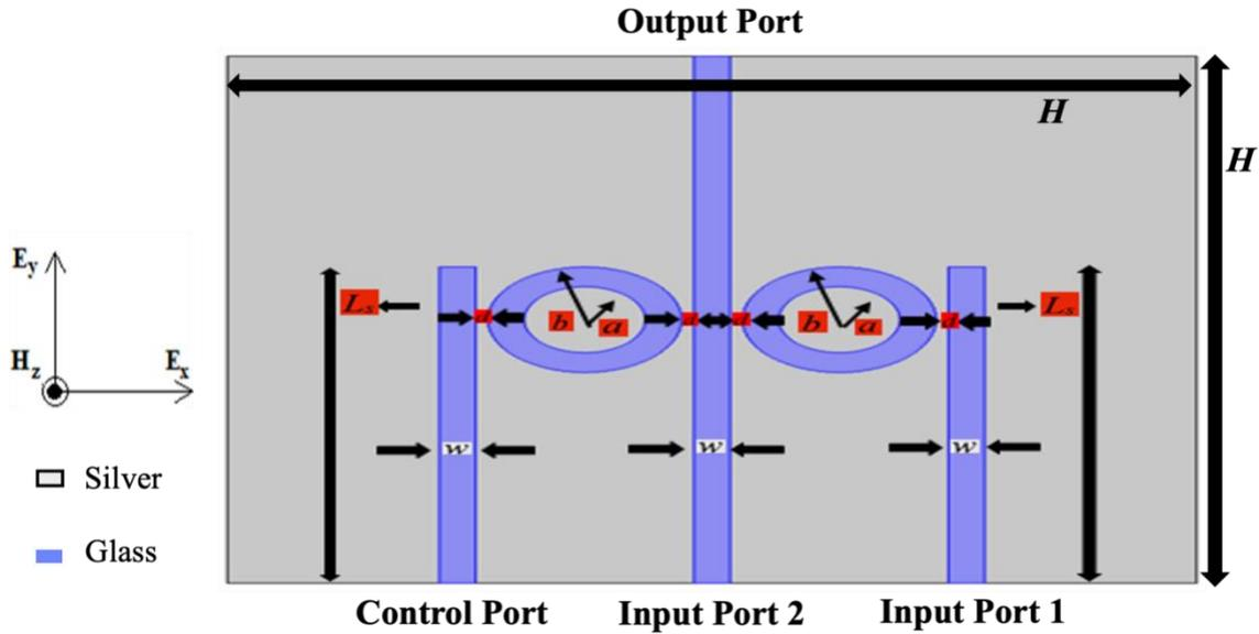
Figure 1 Plasmonic universal logic gates structure
