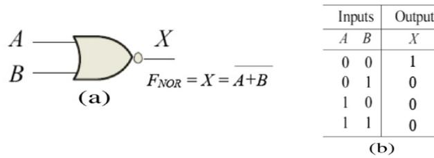
Figure 2 (a) NOR logic gate symbol, and (b) NOR logic gate truth table
