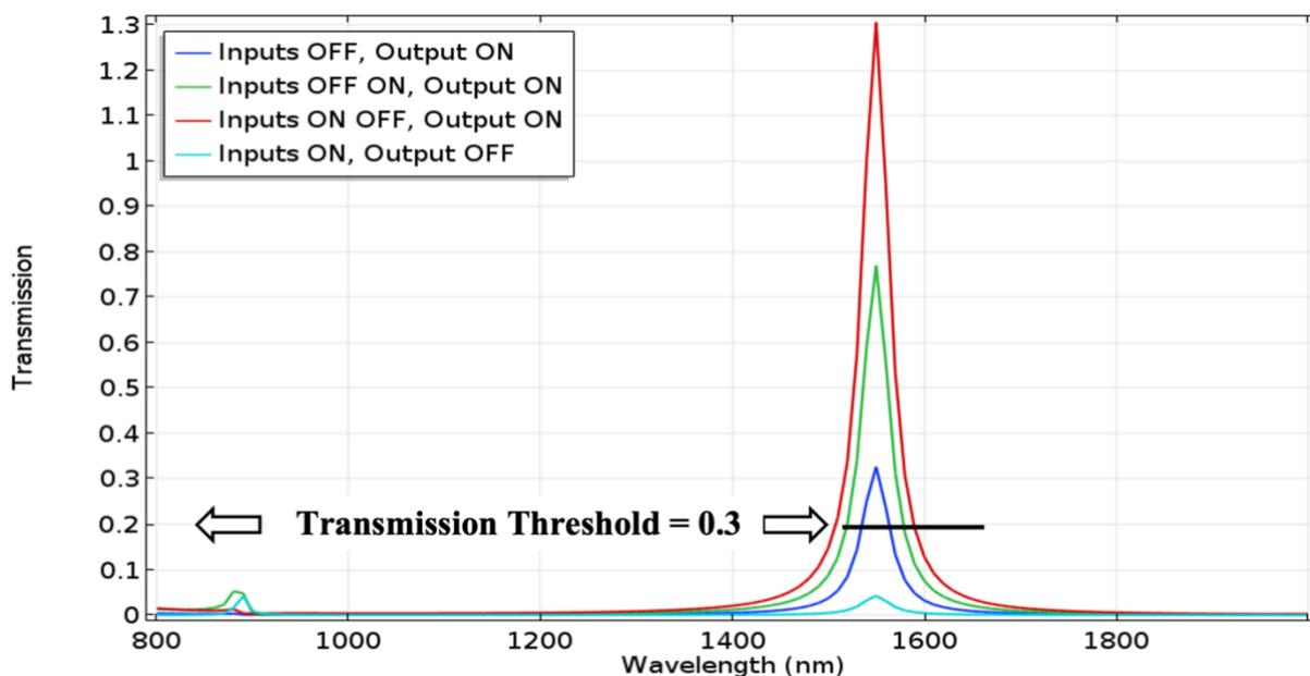
Figure 5 The transmission curve Vs. wavelength range for NAND logic gate
