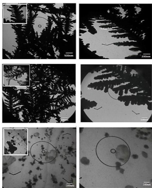
Figure 4 TEM images of Ag nanoparticles prepared at (a) at 80 wt% AgNO 3 and 20 wt% sucrose with preparation time 10 min, (b) at 80 wt% AgNO 3 and 20 wt% sucrose with preparation time 25 min, and(c) at 60 wt% AgNO 3 and 40 wt% sucrose with preparation t
