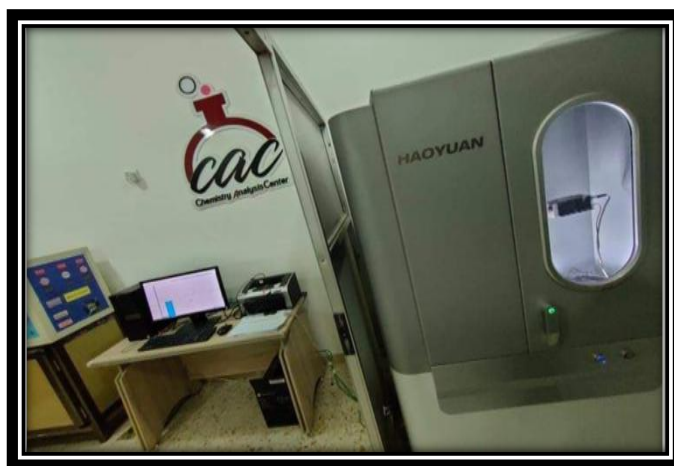
Figure 2: X-ray machine, 2700AB HAOYUAN co., china (4)" The number "4" at the end of the phrase may indicate that this is the fourth X-ray machine produced by this company.
