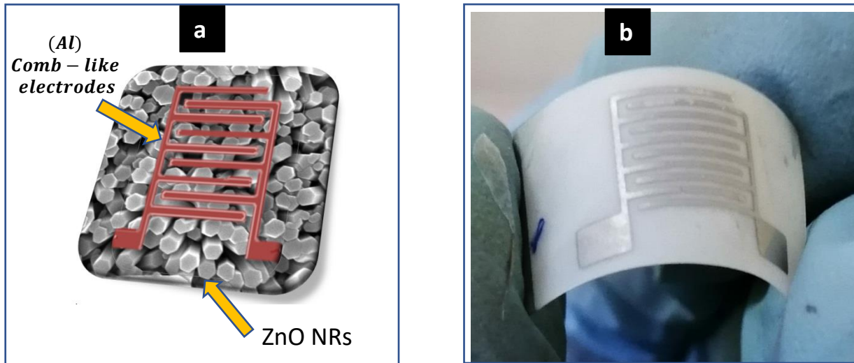
Figure 1. (a) Schematic diagram of Al comb-like electrodes onto the ZnO/PET NRs; (b) Real image of the ZnO/PET photodetector.
